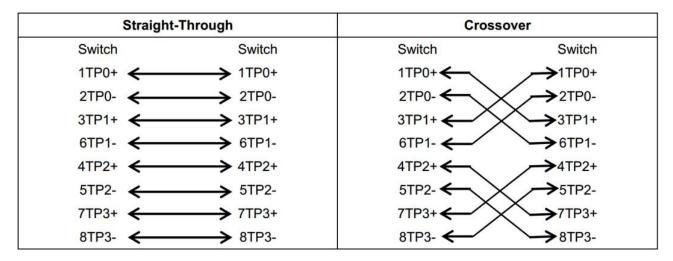
In addition to the preceding cables, the 100BASE-TX/10BASE-T can also use 100-ohm Category-3, Category-4, and Category-5 cables for 10 Mbps, and 100-ohm Category-5 cables for 100 Mbps, both of which can be up to  $100 \, \text{m}$ . Figure A-2 shows the pinouts of the  $100 \, \text{BASE-TX}/10 \, \text{BASE-T}$ .
