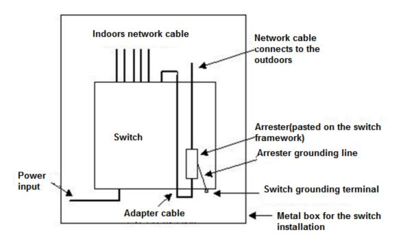
1 The Ethernet port arrester applies to only the 10M/100M electrical Ethernet ports with the RJ45 connector.
