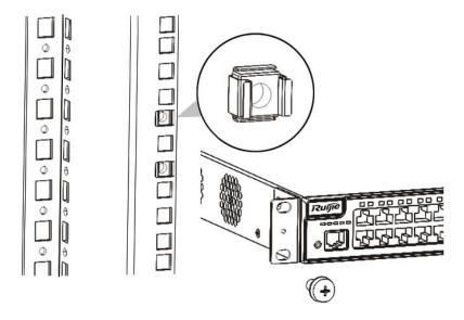
Figure 3-3 Attaching the Brackets to the Rack
