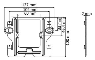
Figure 4-1 Wall Mounting Plate
