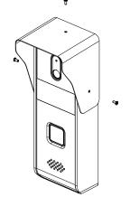
Figure 4-5 Secure Wall Mounting Shield
