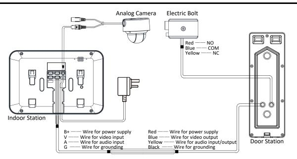
Figure 3-3 Wiring 1 (1 Door Station and 1 Indoor Station)
