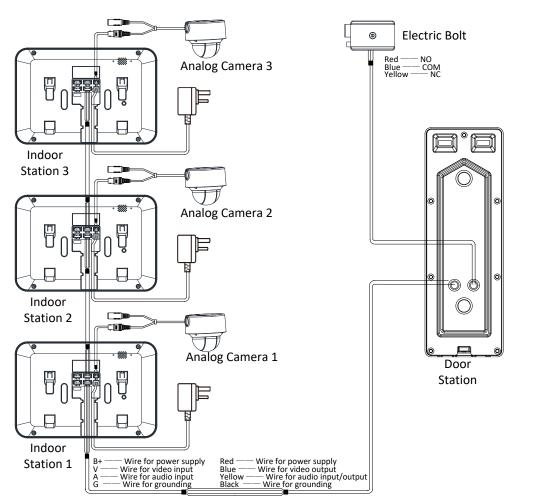
Figure 3-4 Wiring 2 (1 Door Station and 3 Indoor Stations)
