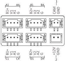
Figure 3-1 Terminals of Indoor Station
