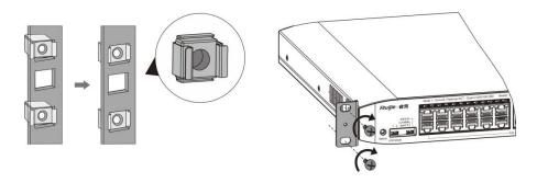
Figure 3-5 Attaching the Brackets to the Rack
