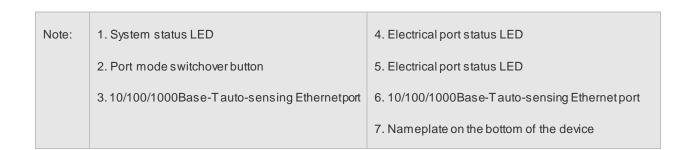
When the button is turned to the left position (Mode 1), the LED indicates the switching status of the port. When the LED is solid green, the link is Up. When the LED blinks green, data is being transmitted or received.
