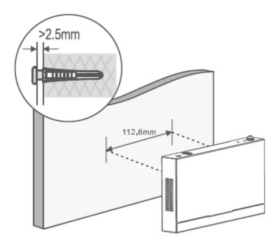
$\triangle$  It is suitable for mounting on the concrete or non-combustible surface only.
