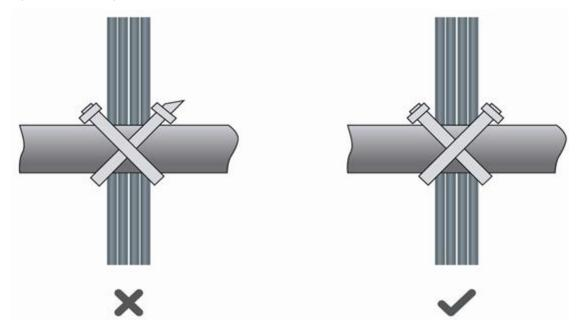
When cables need to bend, first bundle them up. However, the buckle cannot be bundled within the bending area.
