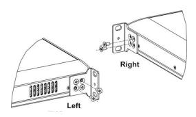
Figure 3-3 Attaching the Mounting Bracket to the RG-ES224GC or RG-ES216GC
