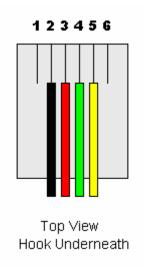
When testing RJ11 phone cables: Tester will test each pin sequentially. Green LED will illuminate for phone cables starting at pin 1 and ending at pin 8. Cable is GOOD when all green LED's light up in sequential test order:
