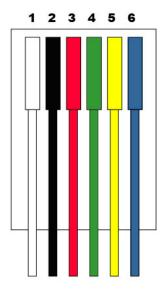
When testing RJ12 phone cables: Tester will test each pin sequentially. Green LED will illuminate for phone cables starting at pin 1 and ending at pin 8. Cable is GOOD when all green LED's light up in sequential test order:
