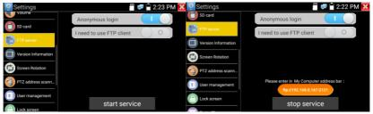
Start the FTP server and then input the tester's FTP address in the PC's address bar. This will enable the PC to read, copy and edit the files from the SD card without the use of SD card reader. **Version information:** Shows applications version information, if press any apps icon several seconds to uninstall.
