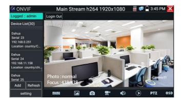
Click the button "Refresh", tester will scan the ONVIF camera again. Click the newly displayed ONVIF camera on the "Device List". The tester will show the IP camera's relative information and settings.
