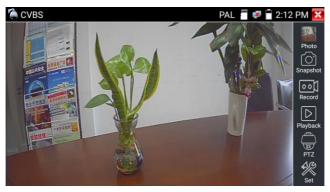
Check and set the protocols, address, interface and baud, all must be consistent with the dome camera, then the IPC tester can test. After setting the parameter, the tester can control the PTZ and lens.
