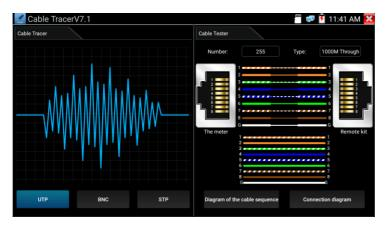
**Note:** If use BNC adapters and alligator clip cable to connect BNC cable etc. Please switch to "BNC mode", if connect shielded cable, please select "STP mode". UTP mode is used for searching the normal network cable or other cables. "BNC mode" for finding BNC cable after connecting adapter. STP mode is used for searching the shielded network cable.
