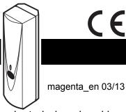
The MAGENTA detector enables detection of plate, tempered or laminated glass breaking. The detector will report the alarm when a low frequency sound (impact) followed by a high frequency sound (glass-break) are registered. The high-frequency channel is analyzed for four seconds from receiving the low-frequency sound wave.
