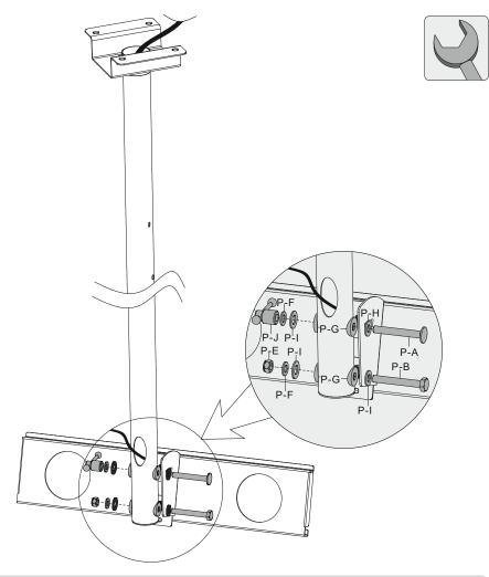
Assemble the universal plate and bottom pipe with connect plate. Using correct combination of screws, washers, nuts and iron knob.
