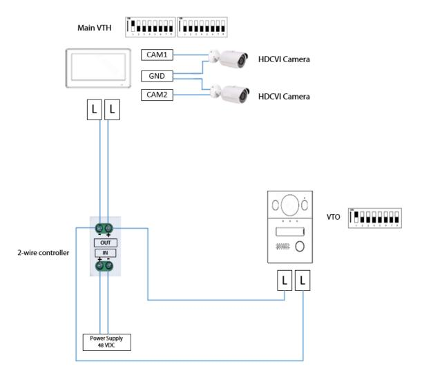
Figure 3-2 Network diagram (with line termination terminal and branch terminal)
