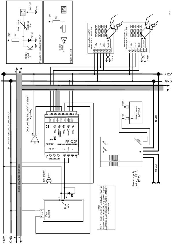
Fig. 2 PR102DR connection diagram
