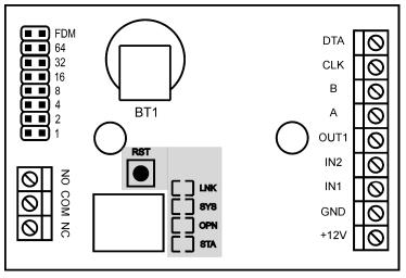
Fig. 4 LEDs at PR102DR-BRD controller PCB
