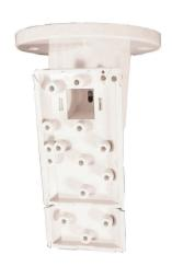
Surface-mount the swiveling B338 plastic ceiling mount to the ceiling. It is suitable for use with many detector types. The vertical swivel range is  $+7^{\circ}$  to  $-16^{\circ}$ , while the horizontal swivel range is  $\pm 45^{\circ}$ .
