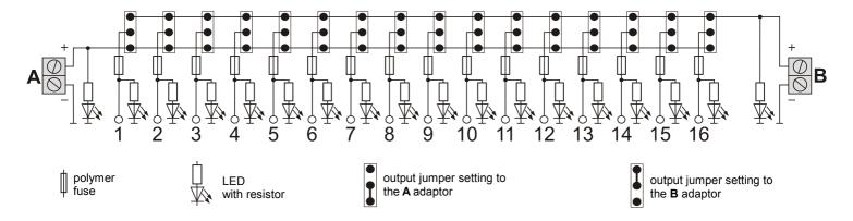
Example of the connection diagram (12 cameras powered with DC 12V, 4 cameras powered with DC 40V):
