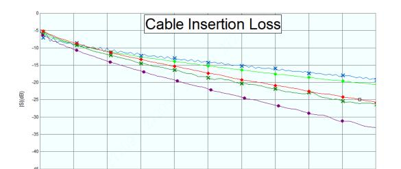
Figure 2-7 Cable insertion loss
