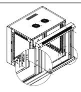
[6] Install front frame by 4pcs of M6\*12 screws (6pcs of M6\*12 screws if more than 18U), refer to the picture.
